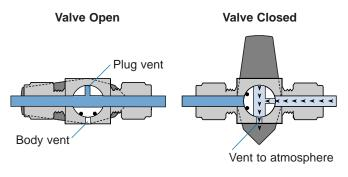
Vented plug and valve body allow pressure release to atmosphere when valve is closed.
